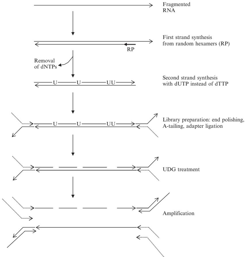
**Figure 5.1** Principle of the dUTP strand-marking ssRNA-Seq method.
